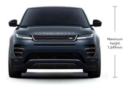
Width 1,996mm mirrors folded Width 2,100mm mirrors out
